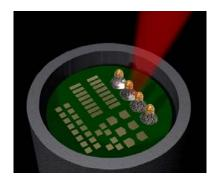
Viable Options: Soldering Iron (at lower production rate) and Diode Laser Best Fit Choice: Diode Laser
