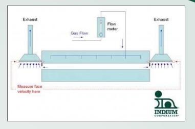
**One final note:** Inert or "nitrogen" soldering really should be renamed "low oxygen level" soldering to place emphasis on the control variable: the ppm oxygen  $(O_2)$ . From an engineering perspective, it IS a critical control variable, and ppm levels within reflow ovens should be measured on a continuous basis.
