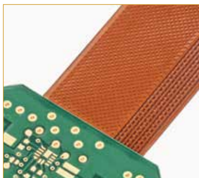
FIGURE 2. This image is a solid plane with round dots removed to provide a cross-hatch pattern.
