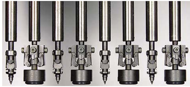
The head assembly has been the object of continuous development and improvement. The photo shows the inline eight-head layout of the 2004 YG100B, with alternating high-precision nozzles for chip placement and nozzles for large or odd-shaped SMDs.
