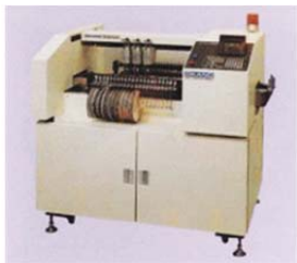
OCM8500 (1984) Compact XY-axis robot-type multipurpose mounter developed for OEM sales.
