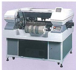
YM6000T (1987) An early Yamaha-brand mounter. Parts picked up by a suction nozzle were mounted on the printed circuit board after positioning by a mechanical centering device.
