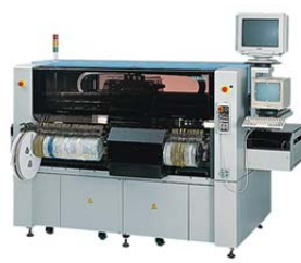
YV112 (1992) Fitted with an inline 16-nozzle multi-head. This was the first model to utilize "full-vision" image processing verification for all SMDs mounted.
