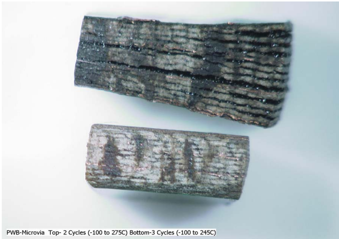
Figure 17 Condition of TMA samples: the top one exposed to one cycles ( -100^{\circ} to +275^{\circ}\text{C} ); the bottom one exposed to 3 thermal cycles ( -100^{\circ} to +245^{\circ}\text{C} ).
