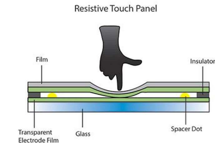
**Figure 2:** Make contact to the resistive touch screens (Source from epectec.com).
