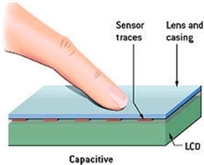
**Figure 3:** Contact being made on a capacitive touch screen.
