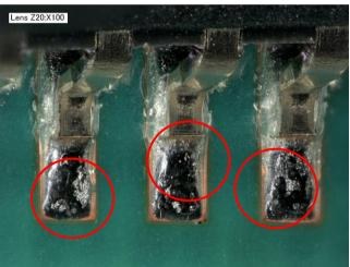
Figure 5: Low-Ag Alloy A - Peak 240°C at 60 sec TAL Uncoalesced/Unreflowed solder paste
