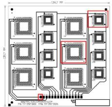
Figure 1: BGA Manufacturing DoE Test Board. Boxed locations (U4, U9, PCB pad for U11) are thermocouple locations.
