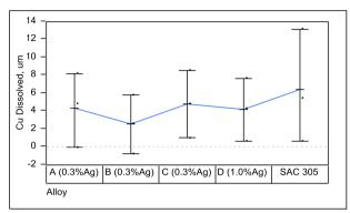
Figure 4: Cu dissolution distribution by alloy
