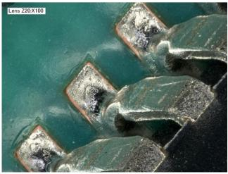
Figure 7: Alloy A – Peak of 240°C at 60 sec TAL Uncoalesced/Unreflowed solder paste
