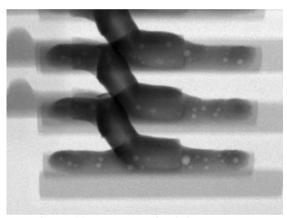
Figure 11: Example of voiding observed
