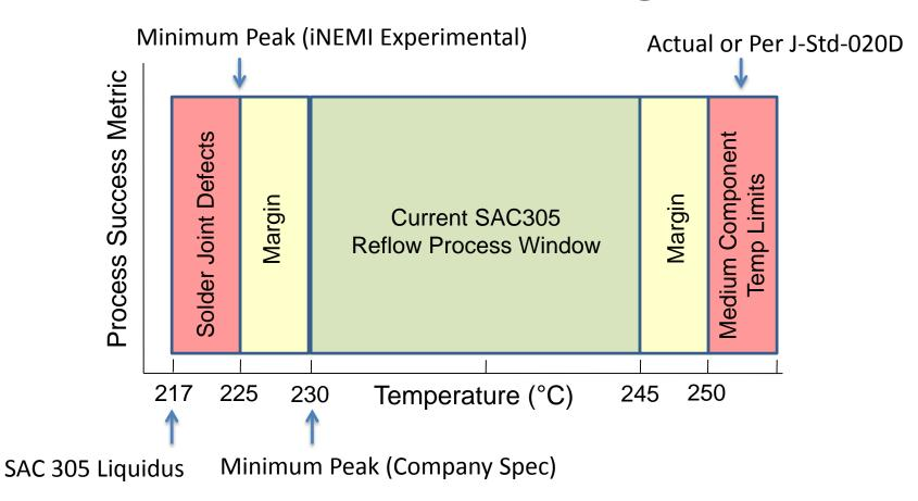
The minimum peak temp for SAC305 is  $\sim$  10-15  $^{\circ}$ C above the liquidus
