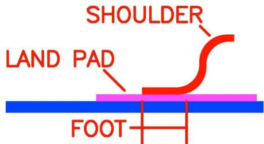
The gull wing lead has a limit as to how much solder volume will wet to the surface. Any excess flows off of the PCB land pad and bridges to adjacent pads, when looking at fine pitch components. The solution is to reduce the volume of solder paste deposited at print.
