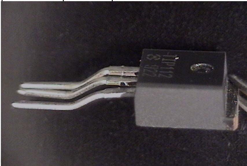
Figure 4-Throughhole to SMT Device Modification of Voltage Regulator (BEST Inc)
