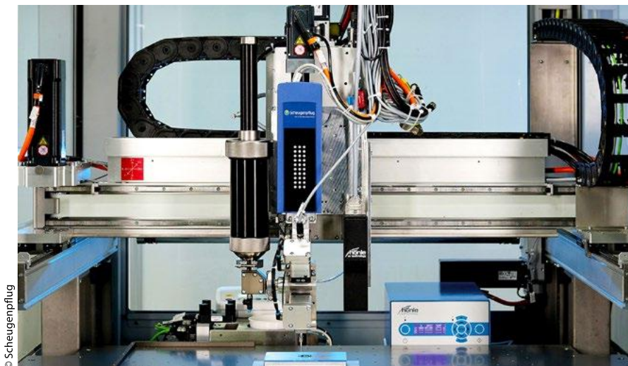
Figure 3 > Dispensing and curing combined in one system
