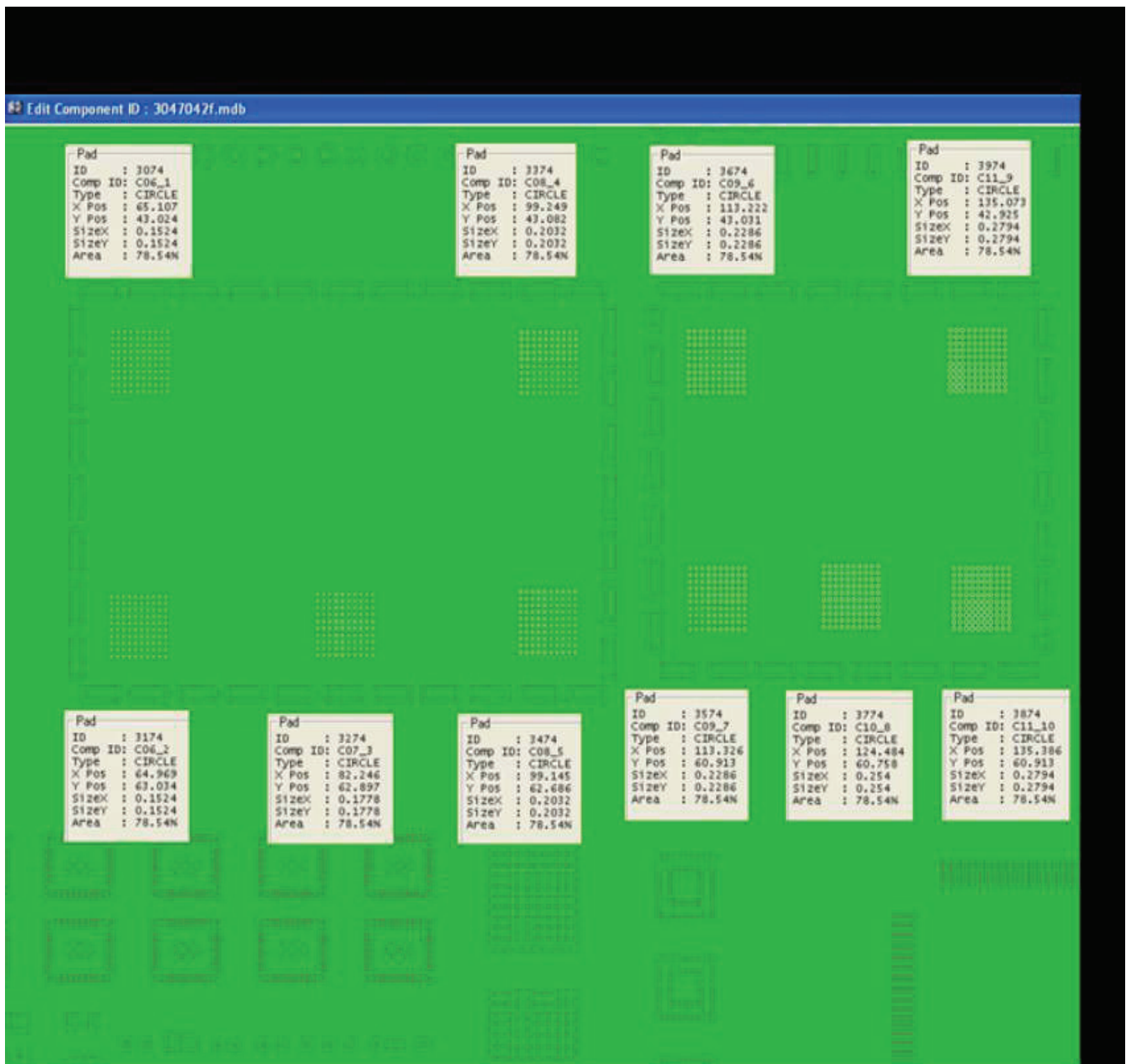
Figure 23 Benchmarker II Board showing test sites for 4 mil (100u) thick stencils: 1,000 total sites per board
