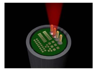
2. Focus the laser spot on the opposite side of the pin from the paste, heating the pin and annular ring. If the surrounding materials are too sensitive to overheating, this process will typically take longer as the heating rate must be slow enough to allow conduction to reflow the solder paste without damaging the surrounding material. The solder will reflow when the pin and ring achieve reflow temperature and run towards the area of highest temperature, where the laser light is focused.
