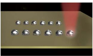
On some products, it is not practical to dispense solder paste everywhere it needs to spread. Applications like pin-in-hole where it is easier to dispense in one spot and heat the product in a way to make the solder paste wet completely around the pin are prime examples. The technique used for these types of joints will vary based on thermal mass and heat sensitivity of surrounding materials. Most work well with one of two options:
