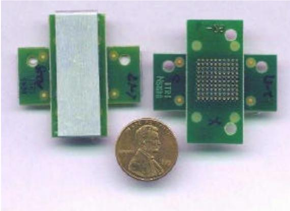
**Figure 13 – TV Coupons Ready for Stress Test**
