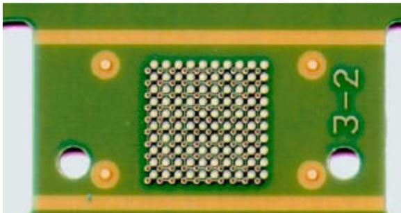
Figure 7 – TV Component Side Coupon Front
