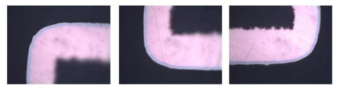
Figure 6, Sample 2 RAI gold (25 minutes dwell time) 5.48 µins gold. No corrosion, Level 0 Product Rating
