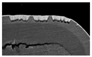
Fig 8 Ni corrosion at 2  $\mu$ in (0.05 $\mu$ m) of phos palladium. Corrosion was extensive and shallow.
