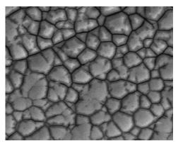
Figure 2 SEM of Ni corrosion
