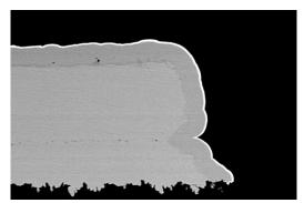
Fig 11. Phos palladium at 2 µins with Reduction Assisted Immersion Gold. Level "0" Corrosion.
