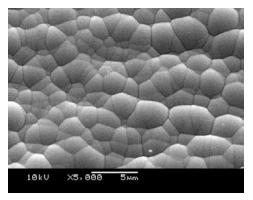
Figure 3 SEM Ni, no corrosion
