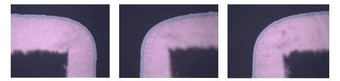
Figure 5, Sample 1 RAI gold 3.12 µins. No corrosion, Level 0 Product Rating
