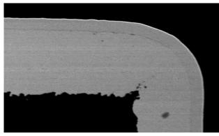
Fig 10. No corrosion at 8.8  $\mu$ in (0.22  $\mu$ m) of phos palladium. No corrosion was found.
