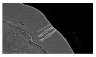
Fig 9 Ni corrosion at 4.8  $\mu$ in (0.12  $\mu$ m) of phos palladium. Few intermittent deep corrosion spikes.
