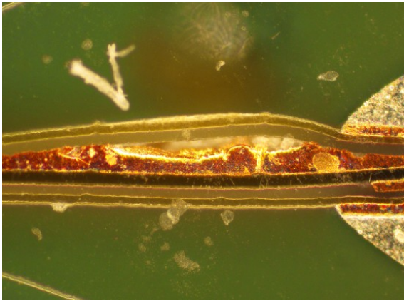
Figure . Cross-section of delaminated pad.
