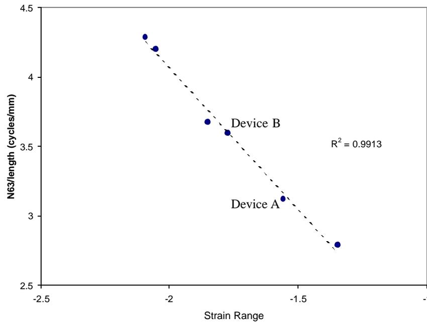
Figure 15. Normalized Characteristic Lifetime versus Strain Range<sup>5,6</sup>
