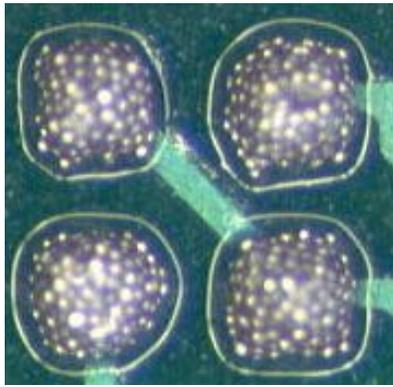
**Figure 4. Type 3 Print Deposits at 0.4mm pitch, Created with .010” Square Apertures, .004” Stencil. Resulting Deposits were “Excessive”.**
