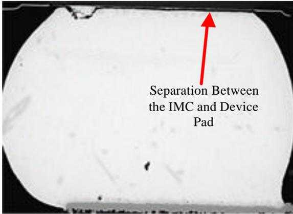
**Figure 14. SnAgCu Failure Due to Separation Between the IMC and Device Attachment Pad. 35 Cycles to Failure.**
