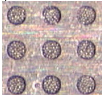
**Figure 6. Clogged Stencil Apertures. Type 4 Paste Screened Over .009” Circular Apertures, .004” Stencil. Third Print between Cleanings.**
