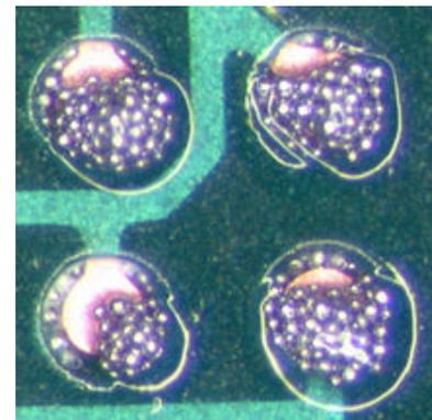
**Figure 3. Type 3 Print Deposits at 0.4mm pitch, Created with .008" Square Apertures, .005" Stencil. Resulting Deposits were Often "Insufficient".**
