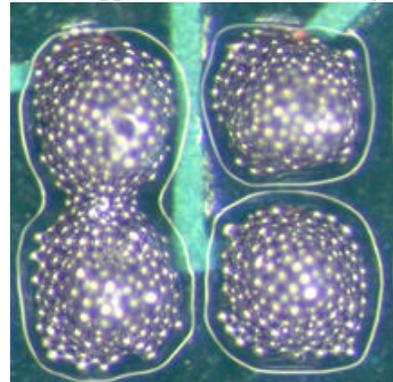
**Figure 2. Type 3 Print Deposits at 0.4mm pitch, Created with .012" Square Apertures, .005" Stencil. Resulting Deposits were Often "Excessive".**
