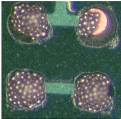
**Figure 5. Type 3 Print Deposits at 0.4mm pitch, Created with .008” Square Apertures, .004” Stencil. Resulting Deposits were Often “Insufficient”.**
