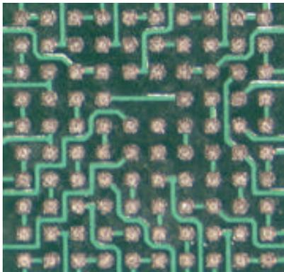
**Figure 8. Type 3 Print Deposits at 0.5mm pitch, Created with .011" Square Apertures, .004" Stencil. No Assembly Defects Observed.**
