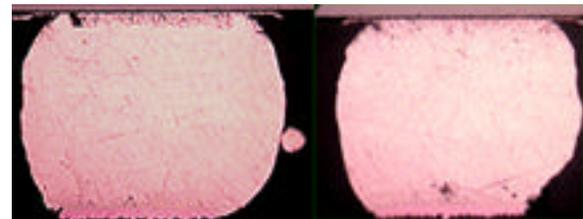
**Figure 9. Cross-sections of Paste Assembled SnAgCu Solder Joints Reflowed in Air. Solder Balls and Irregular Surface Shapes Observed.**
