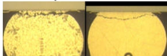
**Figure 12. Typical SnPb (left) and SnAgCu (right) Solder Fatigue Failures Due to Thermal Cycling of Device A.**
