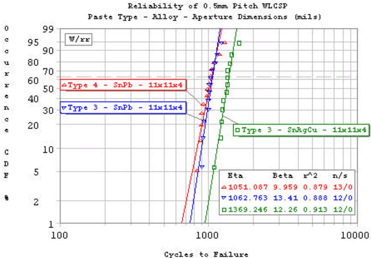
Figure 10. Weibull Plot of 0.5mm Pitch Device B Reliability Data
