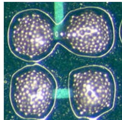
**Figure 7. Type 4 Print Deposits at 0.4mm pitch Created with .010” Square Apertures, .004” Stencil. Deposits are “Excessive” –Resulting in Solder Bridging.**
