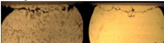
**Figure 11. SnPb (left) and SnAgCu (right) Solder Fatigue Failures Due to Thermal Cycling of Device B.**
