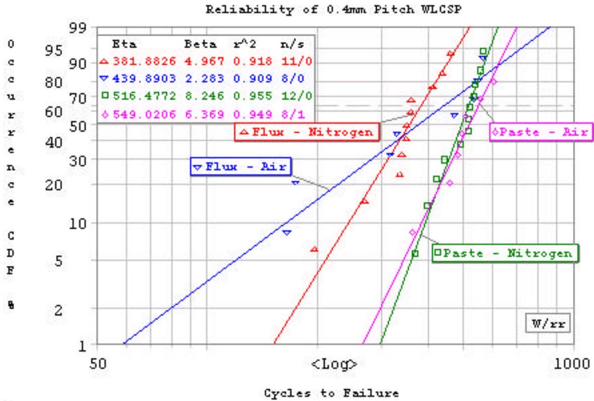
Figure 13. Weibull Plot of 0.4mm Pitch Device A Comparing Reflow Atmosphere
