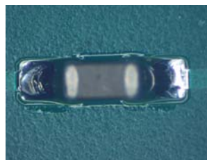
Flux around surface mount
