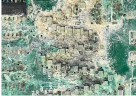
Uncoated PCBA with corrosion
