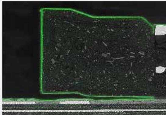
Fig 2: SEM image and chlorine map (combined) of Parylene conformal coating coverage (green line)
