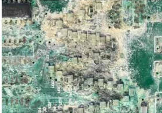
Uncoated PCBA with corrosion
