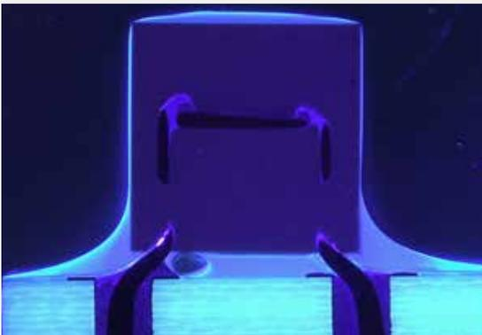
Fig 1: SEM image of conventional conformal coating coverage (Source: IPC-SMTA)
