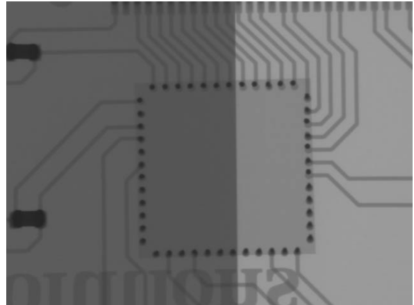
Image J: Image of flip chip with 100 μm thick zinc foil under the left half of the device.
