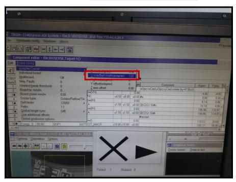
2) Press *Width adjust* button. Now the machine will adjust the belt to the desired size.
