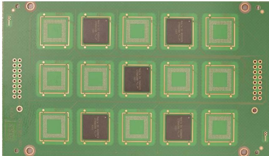
**Figure 11 - Position of components for drop test**
