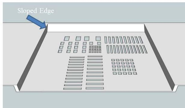
**Figure 7 - Cross section of Step stencil with sloped edge (demonstration)**
