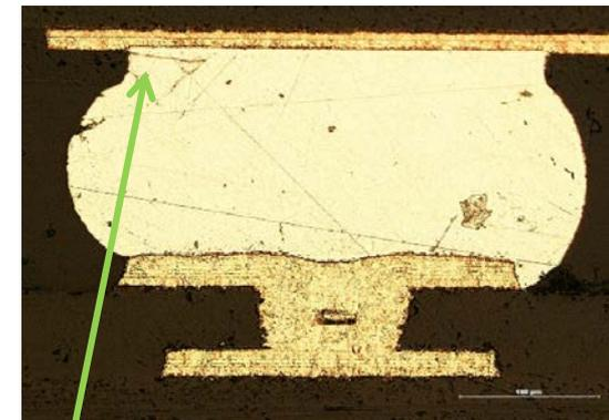
Crack in solder near component
