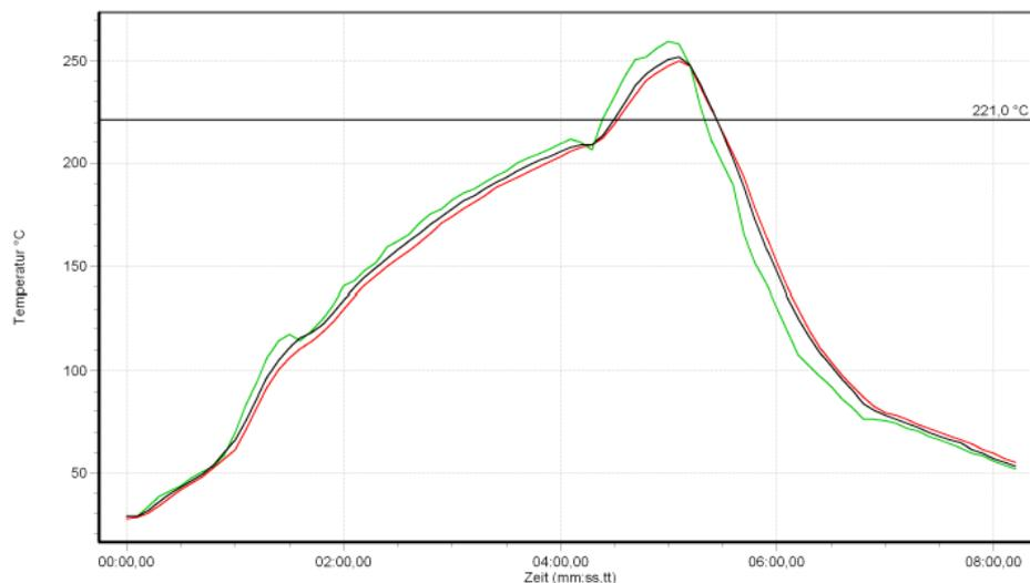
Figure 10 – JEDEC Lead-free Reflow profile
