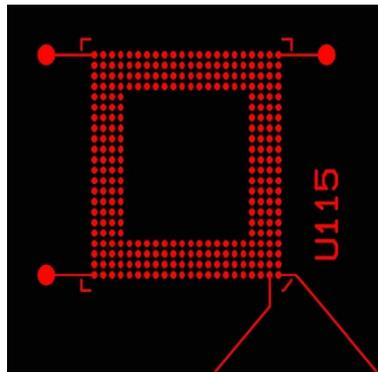
**Figure 1 - Footprint of daisy chain component**
