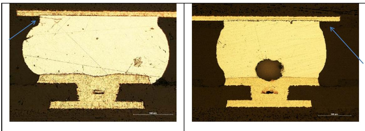
Figure 14 - Crack in solder near component pad
