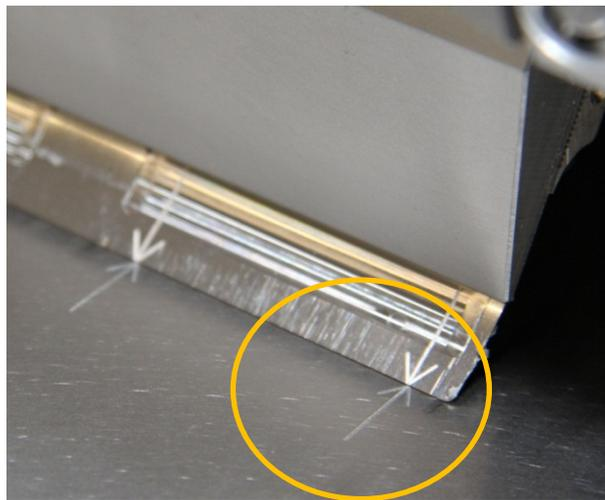
**Figure 8 - Alignment marking on Squeegee and stencil**
