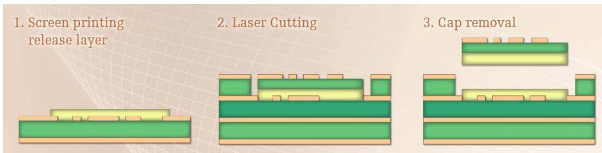
**Figure 3 - Schematic process flow of cavity formation**
