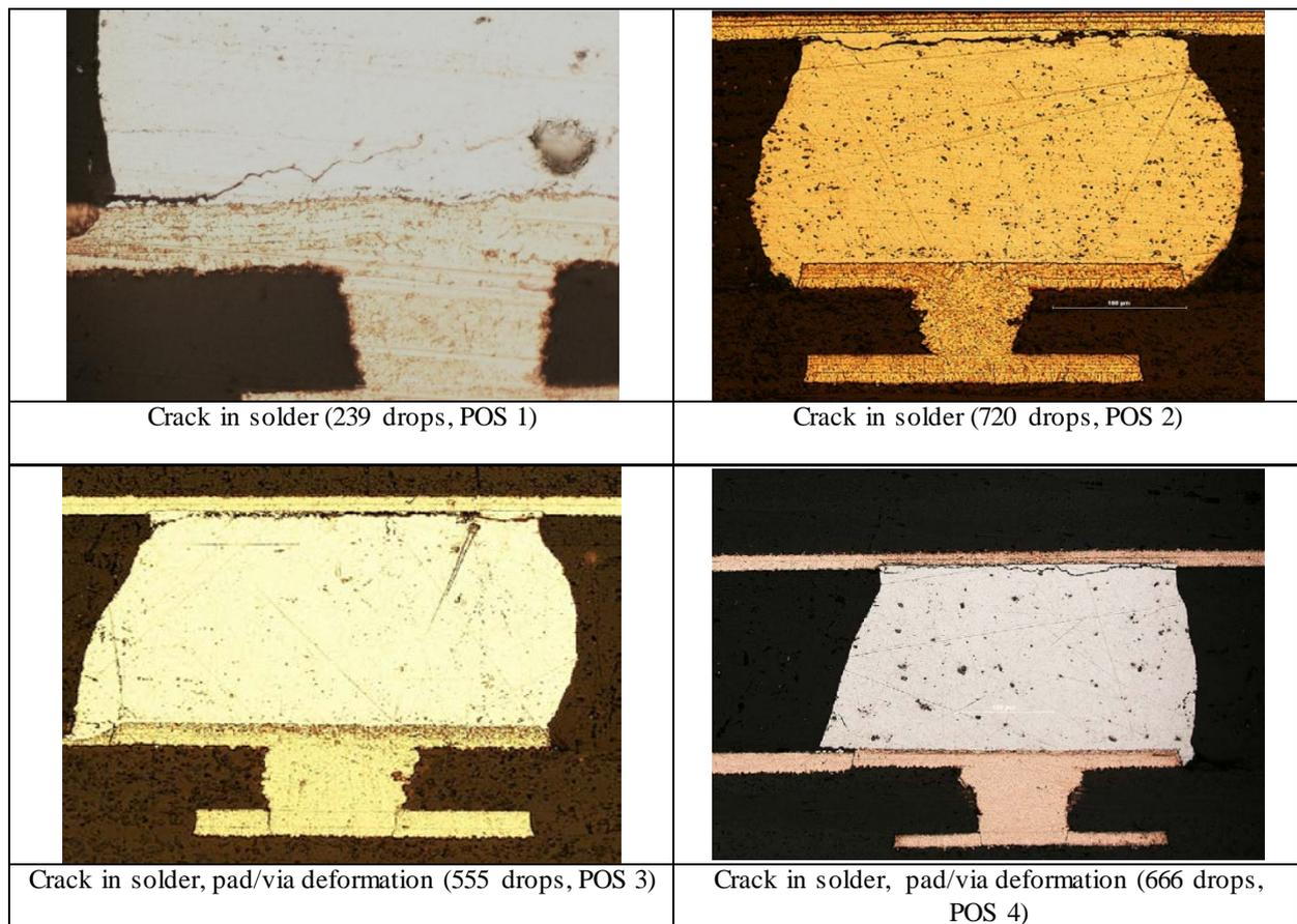
**Figure 16 - Typical failure modes for drop test**
