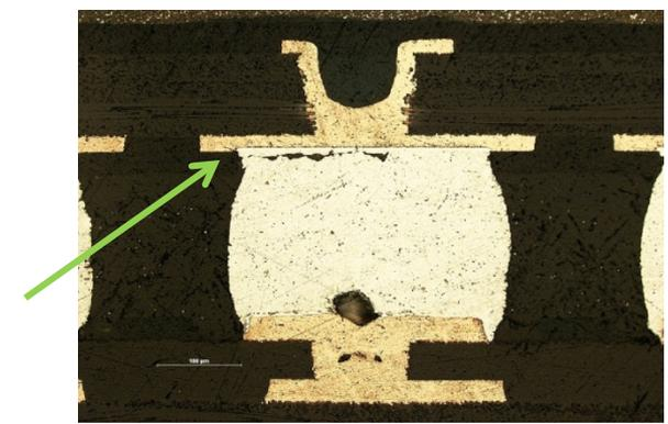
Cracks in solder
