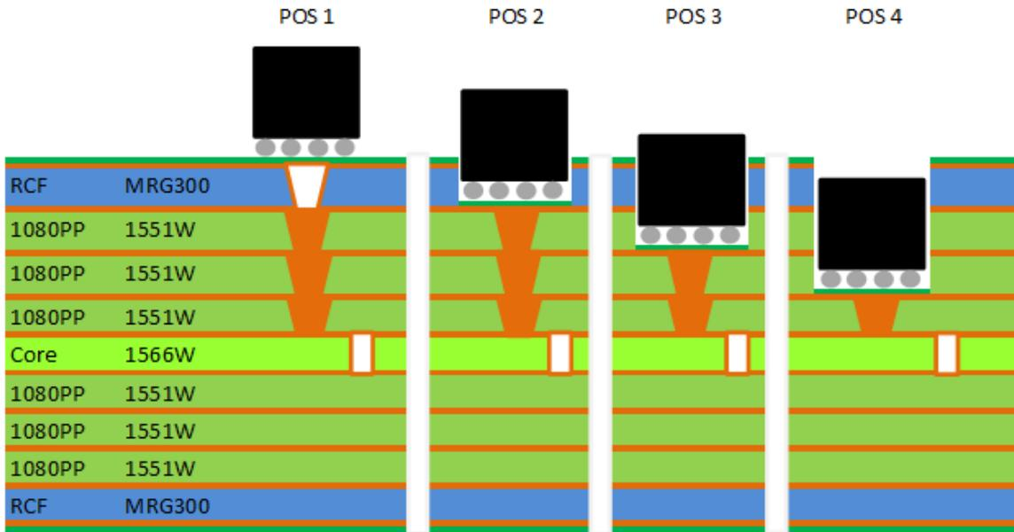
Figure 4 - Test vehicle build-up with recessed areas (PCB and components are not to scale)
