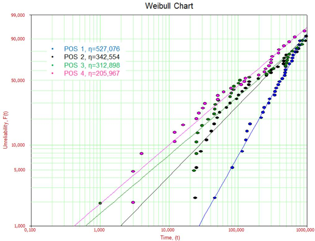
Figure 13 - Weibull chart for all test vehicles (POS 1, POS 2, POS 3 and POS 4)
