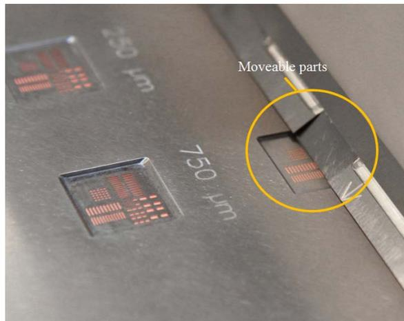
**Figure 6 - Squeegee blade with moveable parts (demonstration)**
