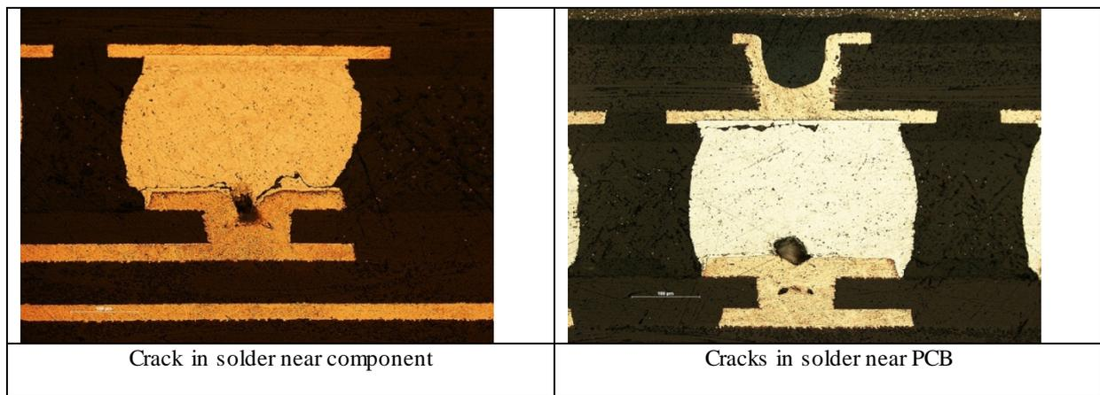
**Figure 20 - Failure modes for TCT**
