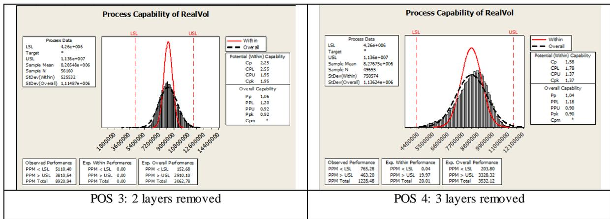
Figure 9 – Process capability of paste volume for all test vehicles (POS 1, POS 2, POS 3 and POS 4)
