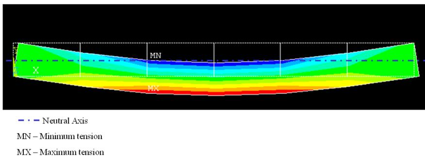
**Figure 12 - Model of tension distribution at drop test**
