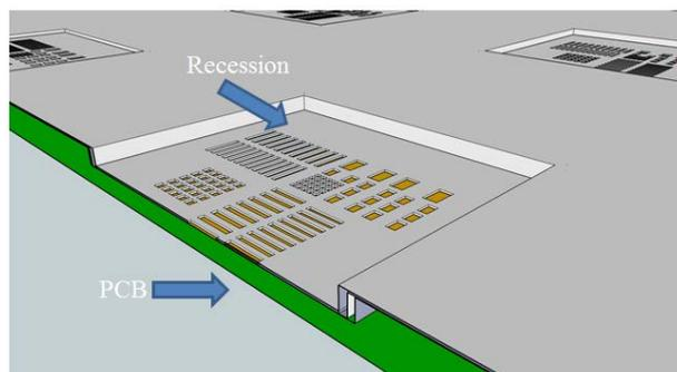
Figure 5 - Overview Step Stencil on PCB (demonstration)
