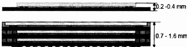
Figure 23 Schematic diagram of a stacked package. [3, 5]
