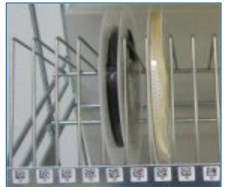
Figure 5. The storage area should have 2D barcodes that should be scanned before any reel is removed or replaced into the storage rack.
