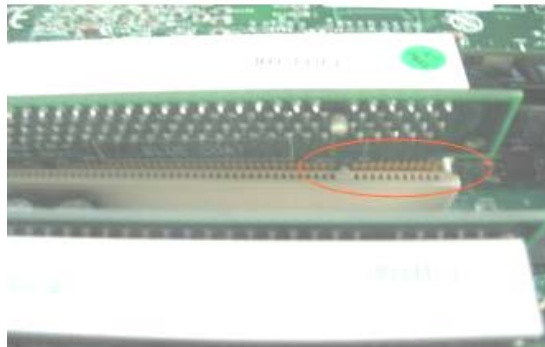
Figure 1 - Example of partial loose contact of Daughter Card from Press-Fit Connector
