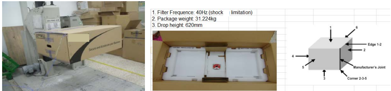
Figure 11 – Lab ten corner-edge-face multiple drop tests to emulate transportation stress
