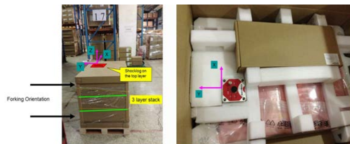
Figure 10 – A shock gravitational force measurement device is embedded in the shipping box
