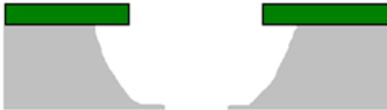
Single-side etching – formation of „knife-edge”
