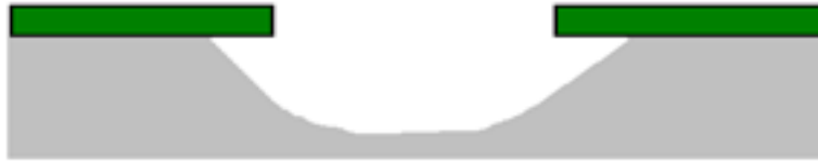
Single-side etching – high degree of undercutting
