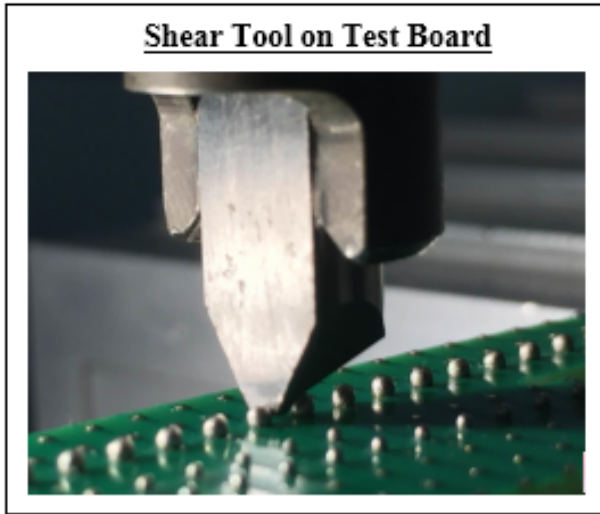
Figure 3. Shear tool on Test Board
