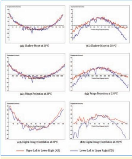
Figure 5. Diagonal plots of a 14mm PBGA at 26°C and 250°C
