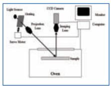
Figure 3. Fringe projection configuration
