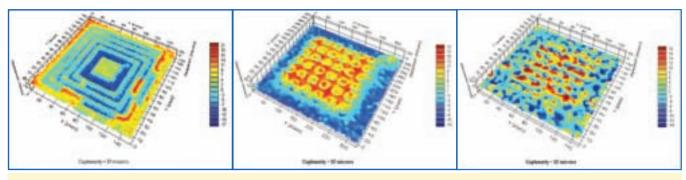
Figure 7. 3D surface plots of a 14mm PCB BGA site at room temperature (a) shadow moiré, full view (b) fringe projection, zoomed view (c) digital image correlation, zoomed view
