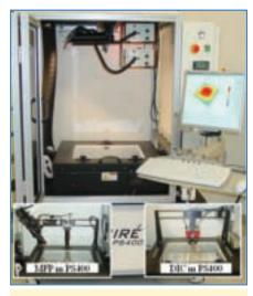
Figure 1. TherMoiré® PS400 with MP10 and DIC set-up
