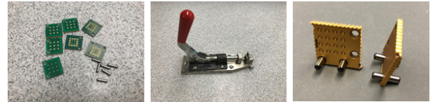
Figure 5: Coupons are loaded on to the pins with the aid of the Pin Loader
