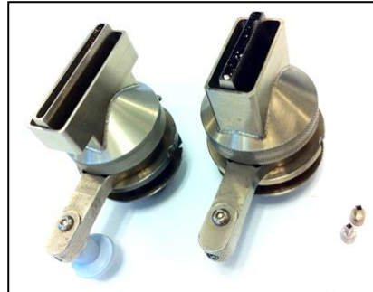
Figure 15. Large Site Cleaning Nozzle (Zevac AG)
