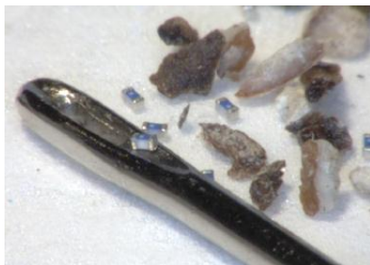
Figure 5. 01005 in eye of Needle and Next to pepper flakes
