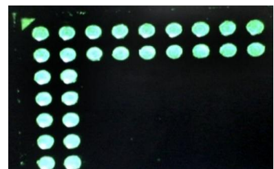
Figure 18. Inspecting Paste on Spheres in Vision
