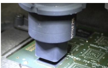
Figure 12. Standard Nozzle (Removes 1 Package at a time)
