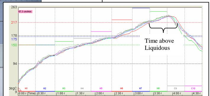
Figure 16 - Resulting Time / Temperature Reflow Profile
