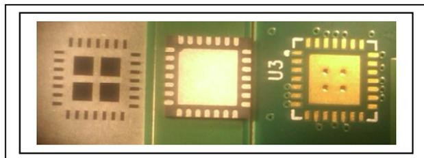
Figure 10 – Stencil, QFN, PCB pattern
