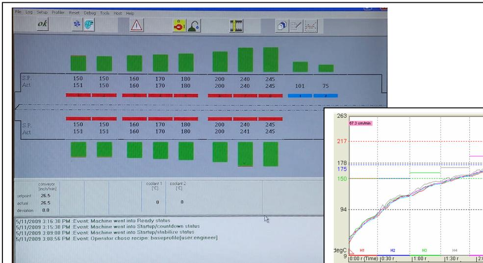
Figure 15 - Reflow Oven parameters. Settings of temperature and conveyor speed
