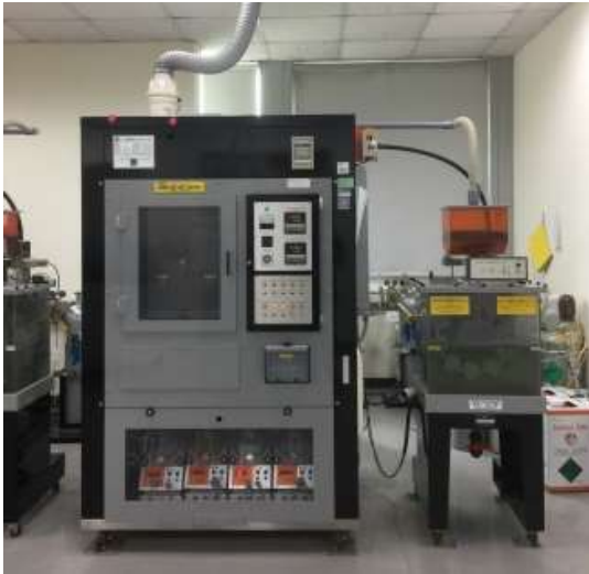
Figure 2.2: Typical mixed flowing gas (MFG) chamber and flowchart
