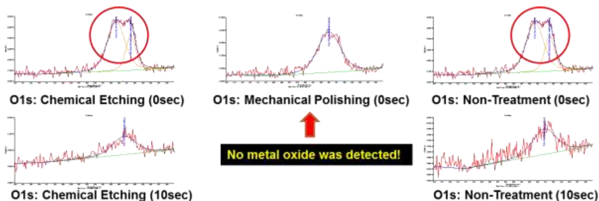
Figure 4.1: XPS results for silver foil with various pre-treatments. Chemical etching did not get rid of the surface silver oxide present on non-treated silver. The oxide could be removed by a 10-second sputter etch. Mechanical cleaning removed the surface silver oxide.
