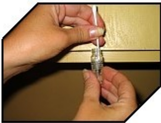
Figure D- Swab on style reagent uses color to tell the user about the presence of lead
