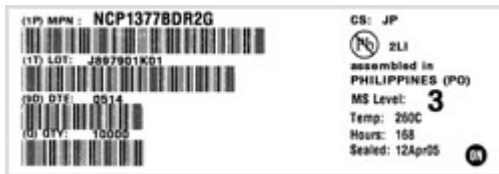
Figure F- Typical lead free component labeling scheme
