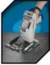
Figure E- Handheld XRF tester provides good level of “first defense” in RoHS compliance and due diligence
