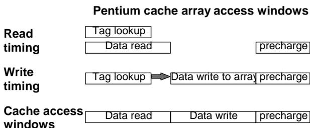
Figure 3. Pentium Processor's Cache Array Access Windows
