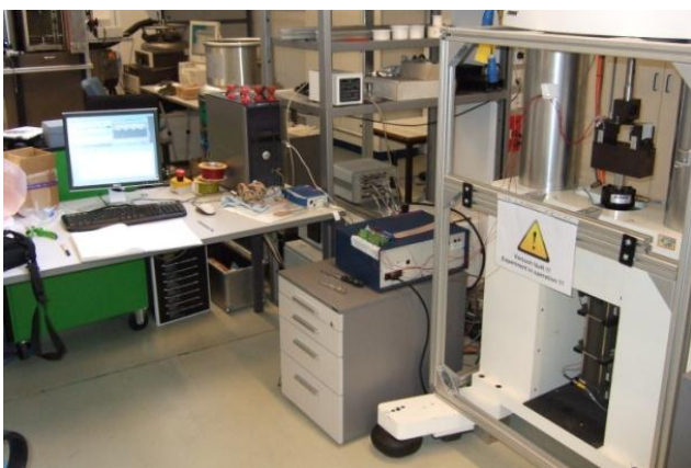
Fig. 7 - Board Level Cyclic Bend Test Set-Up
