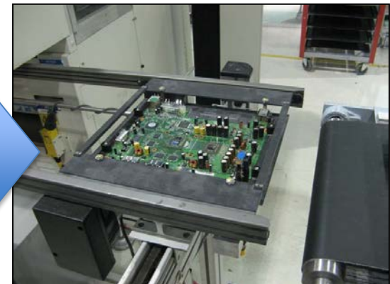
Exit area (Pallet in Down position)
