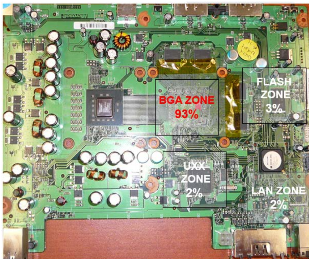
BGA Rework defect concentration diagram
