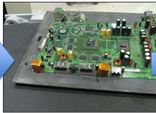
Place extra covers for sensitive TH connector
