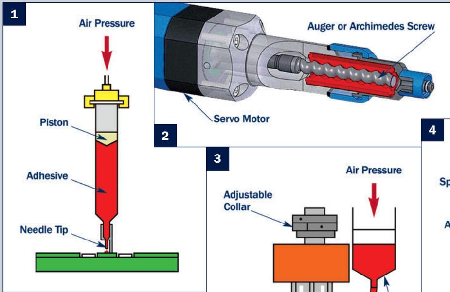
Figure 1: Time-Pressure Valve. Courtesy of EFD, Inc.
