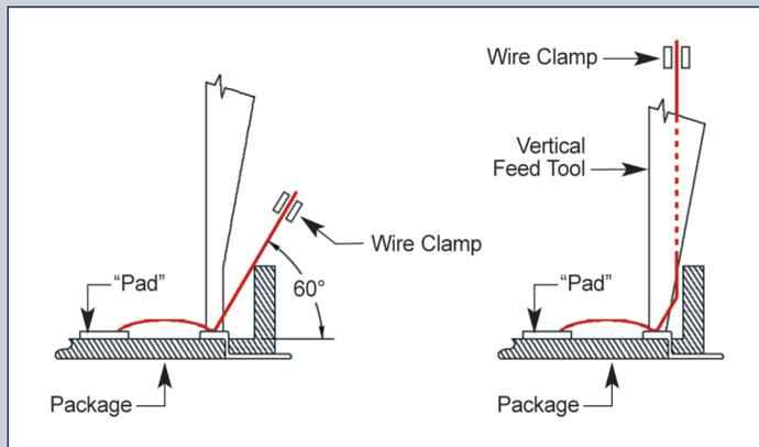
Figure 1: Wire feed angles of 60° and 90°.
