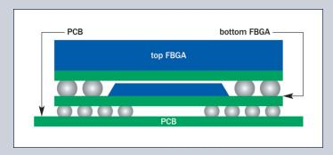
Figure 2: Schematic of POP assembly using FBGA.
