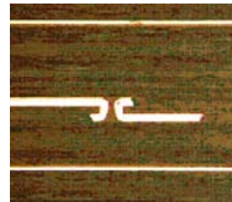
Photo 3. Laser Processed Ultra-small Diameter VIA
