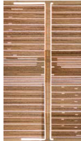
Photo 4. Cross-sectional View of an 80-layer Board
